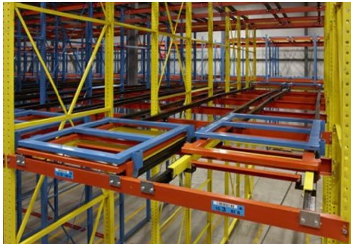
Figure 7. Push-back Racking System [15]
