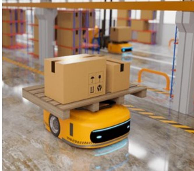
Figure 5. Automated Guided Vehicles (AGVs) [8]
