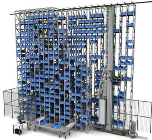
Figure 13. Mini-load ASRS [27]
