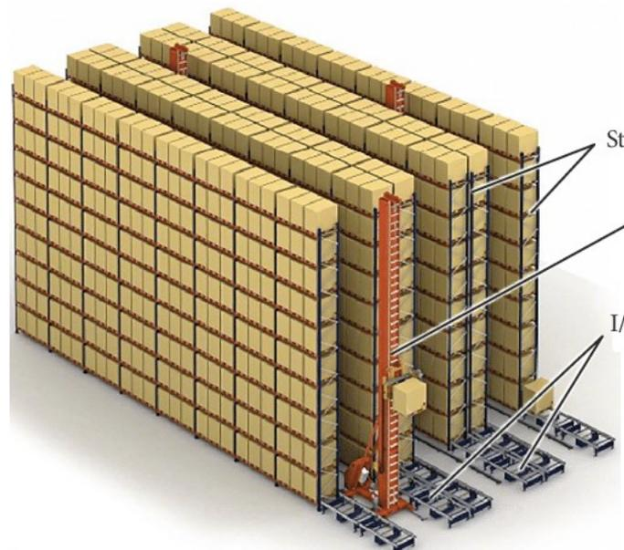
Figure 11. Unit-load ASRS [22]
