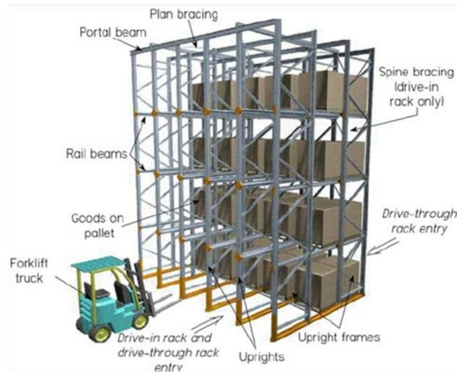
Figure 8. Drive-in and Drive-through Racks [16]
