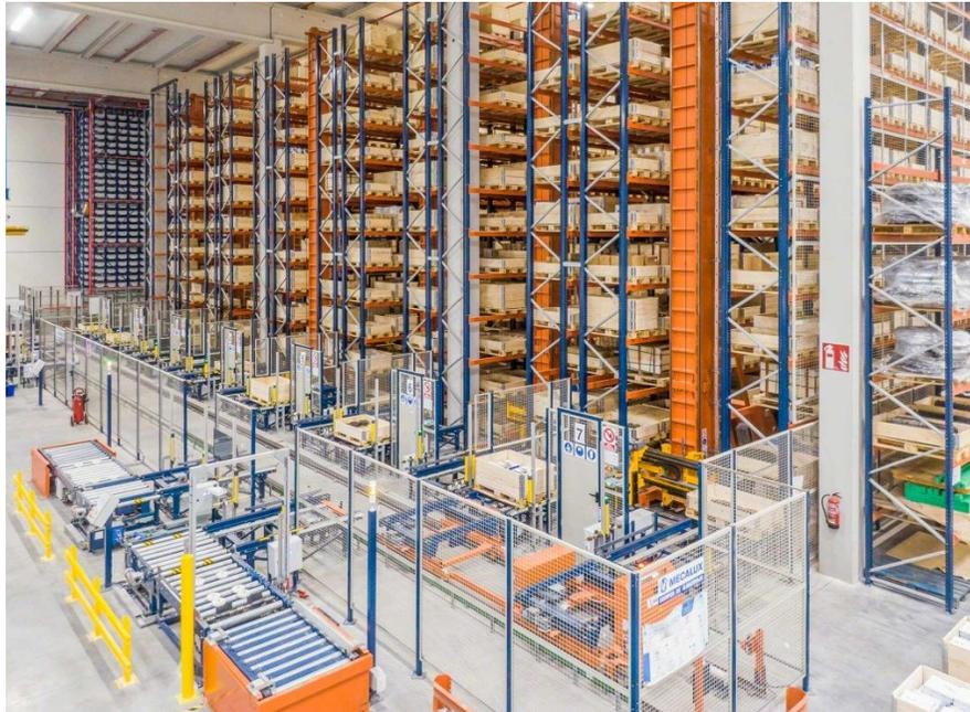
Figure 10. Example Photo of Warehouse with ASRS [18]
