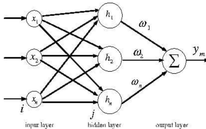
Figure 1. Radial-basis Function Neural Network (RBFNN)
