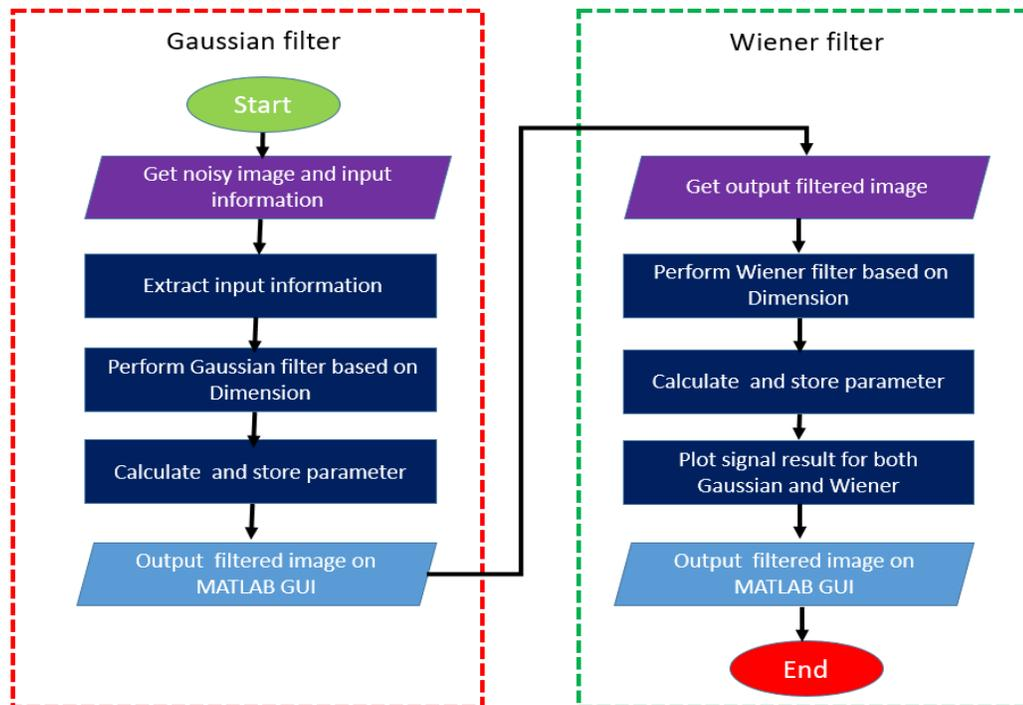
Figure 1. Flowchart of Adaptive Wiener and Gaussian Filter
