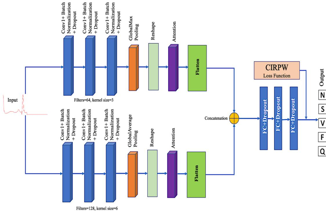
Figure 7. The proposed cost-sensitive dual 1D-CNN with Attention Network
