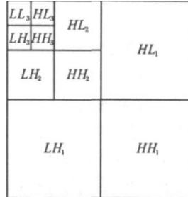
Figure 1. The diagram of three-level wavelet decomposition
