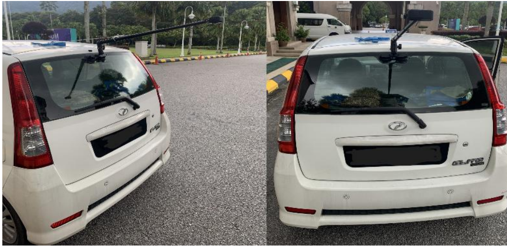
Figure 2. Vehicle-mounted Camera Setup
