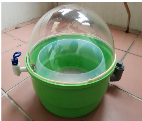
Fig. 8. The complete prototype design of the hemisphere flat based solar still structure.
