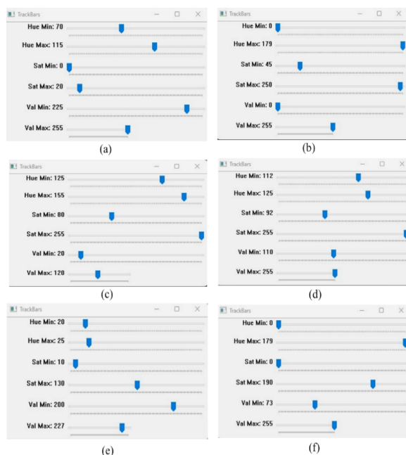
Fig. 36. HSV value on Hue (min) , Hue (max) , Sat (min) , Sat (max) , Val (min) and Val (max) on RM10 (a) Watermark Portrait, (b) Perfect See-through Register, (c) Color Shifting security flat position, (d) Color Shifting security tilt position (e) Colored Glossy Patch and (f) Text, Logo, and Two Color Fluorescent Element.
