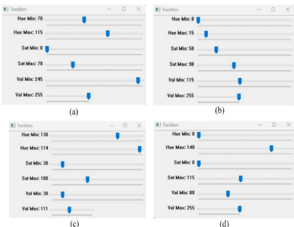
Fig. 54. HSV value on Hue(min), Hue(max), Sat(min), Sat(max), Val(min) and Val(max) on RM50 (a) Watermark Portrait, (b) Color Shifting security flat position, (c) Color Shifting security tilt position and (d) Text, Logo, and Two-Color Fluorescent Element.
