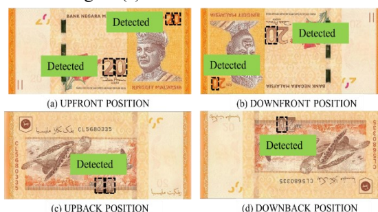
Fig. 15. The possible four inserted Position of RM50 into the banknote reader.
