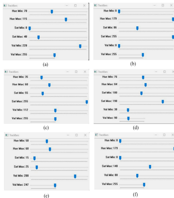
Fig.45. HSV value on Hue(min), Hue(max), Sat(min), Sat(max), Val(min) and Val(max) on RM20 (a) Watermark Portrait, (b) Perfect See-through Register, (c) Color Shifting security flat position, (d) Color Shifting security tilt position (e) Colored Glossy Patch and (f) Text , Logo, and Two Color Fluorescent Element.
