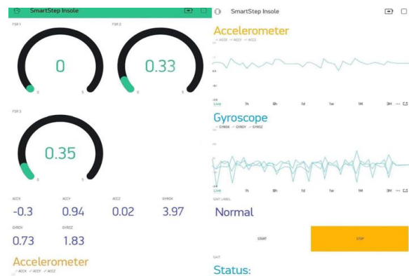
Fig. 5. Blynk interface consists of FSR Sensors Pressure, Accelerometer, Gyroscope, On and Off Button.
