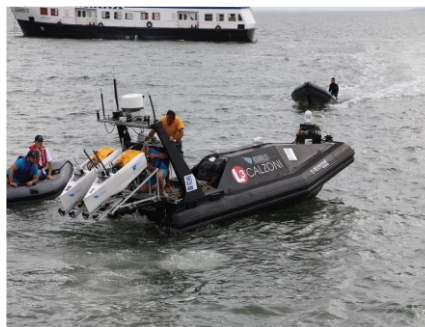
Fig. 10. Two UCAPs mounted on the deployment system installed on the U-RANGER [20].
