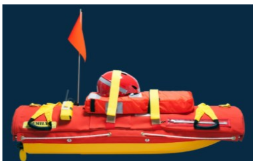
Fig. 13. Rescue and safety equipment in EMILY [22].
