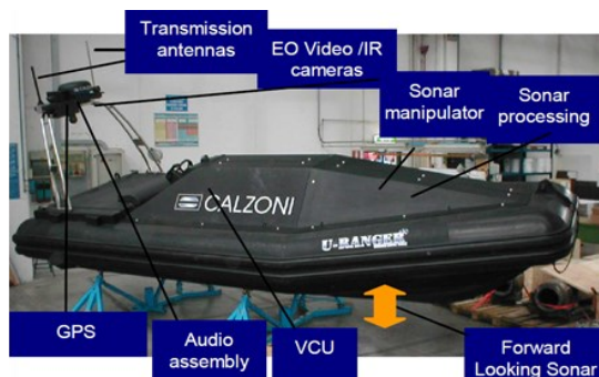
Fig. 6. Allocation of sensor in U-Ranger [18].
