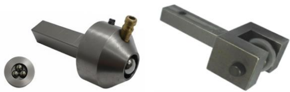
Fig. 2. Ball burnishing tool (left) and roller burnishing tool (right).
