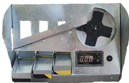
Fig. 10. Physical prototype of the coin sorting machine.
