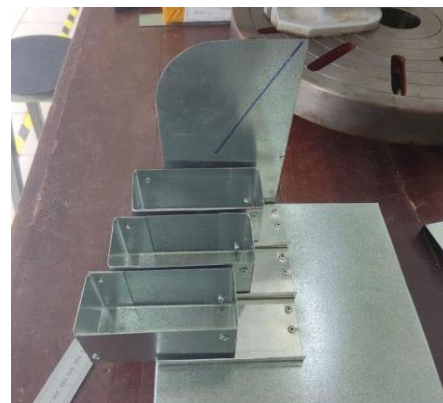
Fig. 8. Container part for the coin sorting machine.
