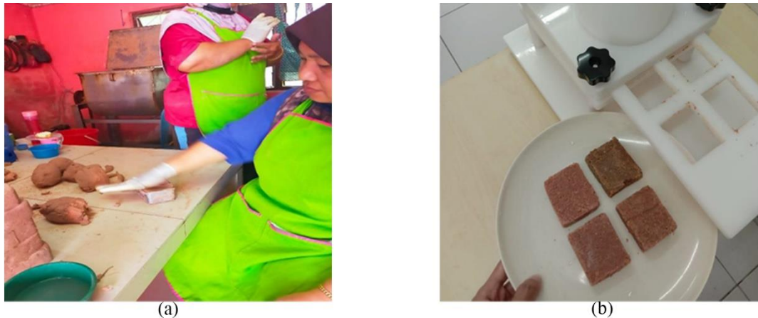
Fig. 7. Shrimp paste moulding process using (a) traditional method and (b) proposed moulding tool.
