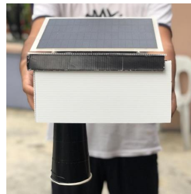
Fig. 5. A Flash Flood Warning System with a solar panel at the top and a pipe with the ultrasonic sensor at the bottom.
