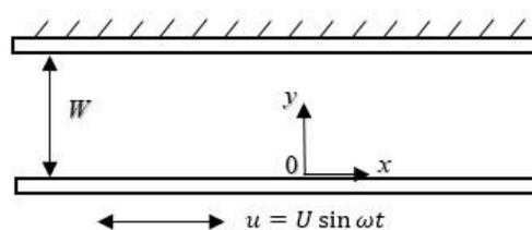
Fig. 1. Schematic diagram for the fluid flow induced by lower oscillatory plate.
