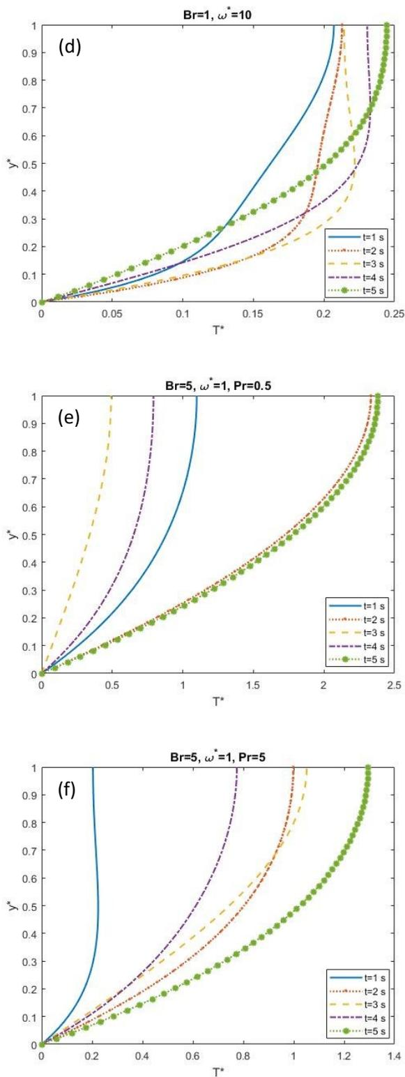
Fig. 4. Fluid temperature profiles in the microchannel induced by the oscillatory flow at (a)  $Br = 5$ ,  $\omega^* = 1$ ,  $Pr = 1$ , (b)  $Br = 10$ ,  $\omega^* = 1$ ,  $Pr = 1$ , (c)  $Br = 1$ ,  $\omega^* = 5$ ,  $Pr = 1$ , (d)  $Br = 1$ ,  $\omega^* = 10$ ,  $Pr = 1$ , (e)  $Br = 5$ ,  $\omega^* = 1$ ,  $Pr = 0.5$ , and (f)  $Br = 5$ ,  $\omega^* = 1$ ,  $Pr = 5$ .
