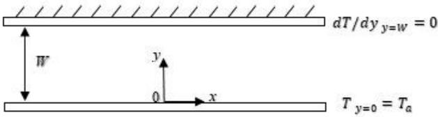
Fig. 2. Schematic diagram for the thermal boundary conditions in the microchannel oscillatory flow.
