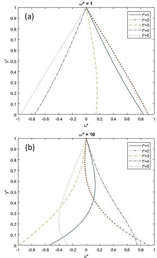
Fig. 3. Two selected velocity profiles in the microchannel induced by the oscillatory flow at (a)  $\omega^* = 1$  and (b)  $\omega^* = 10$ .
