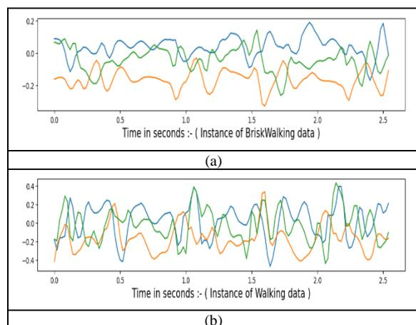
Fig. 7. Gyroscope signal patterns of a (a) brisk walking sample and (b) walking sample.
