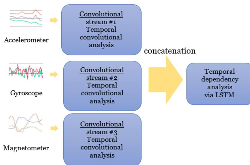
Fig. 1. The overview of the proposed Multi-stream TC-LSTM architecture.
