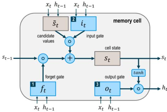
Fig. 5. LSTM memory cell structure (source: Giang *et al.*, 2022).
