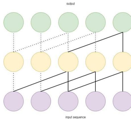
Fig. 4. Dilated causal convolution with two layers with kernel length 2 and dilated rate 2.
