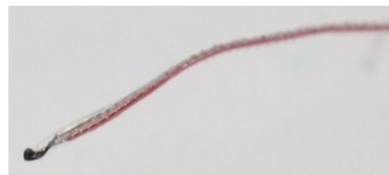
Fig. 2. Welded Type – J thermocouple.
