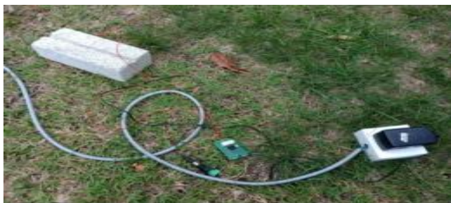
FIGURE 10(E). The perimeter wire connected to the 555 timer signal generator.
