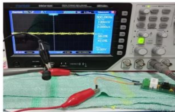
FIGURE 4. The inductor when close to the perimeter wire (no amplification).
