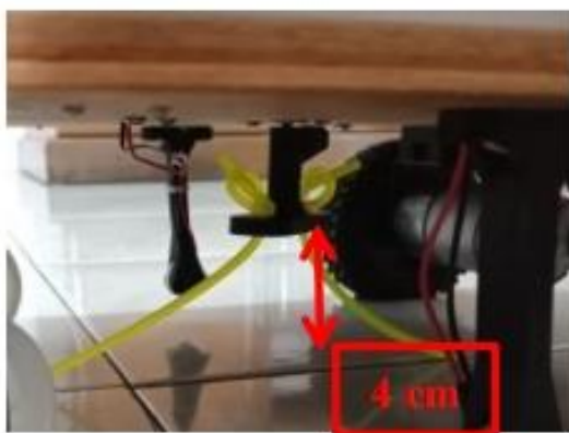
FIGURE 8. The trimmer head of the machine.
