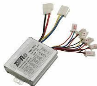
FIGURE 3. Brushed Motor Controller
